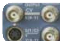
3 Outputs, 1 Y/C (S-Video), 2 Composite, Preview and Composite Outputs may be assigned as (Y/R-Y/B-Y) Component Out
