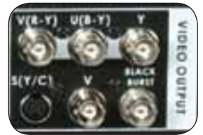
Video Outputs Component, Y/C (S-Video), Composite Video.
