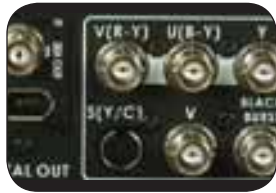
Video Outputs DV (DV25), Component, Y/C (S-Video), Composite and SDI.
