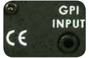
GPI Input Controls preprogrammed EFX F01 to F30 in sequence.
