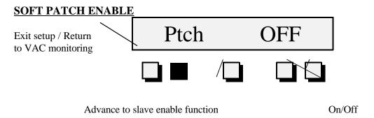
This function enables or disables soft patching. Ptch "off" enables the dimmer channels to be assigned in groups of either 3, 6, or 12 (D360dx / D625dx / D125dx) using a starting address for the first dimmer channel. Ptch "on" allows full soft patching, i.e.: any dimmer channel may be patched to any DMX channel. Soft-patch on memory pages 1 - 5 only. ALSO SEE "DIMMER CHANNEL ASSIGNMENTS".
