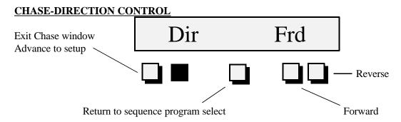
This is the last parameter in the chase menu which determines the initial direction of the sequencer loop i.e.: the first look to the last look ( $\mathbf{Frd}$ ) or the last look to the first look ( $\mathbf{bAc}$ ). Depressing one of the buttons on the right changes direction of the chase. The center button returns to the main sequencer program select menu.
