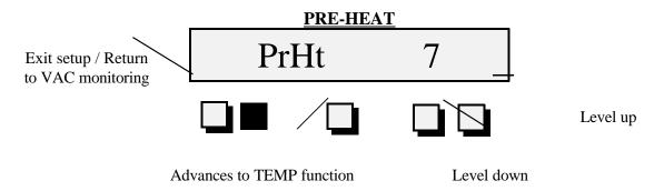
The Pre-Heat function is enabled / disabled via the main menu. In this SETUP menu preheat levels can be programmed from 4 to 10 VAC if the factory pre-selected level of 7 is undesirable, using the level up and down buttons select the desired pre-heat level. The above display indicates all channels will receive a 7% control level for pre-heat when operating on a 120VAC power grid. When operating on a 230VAC power grid maximum preheat level will be slightly higher.
