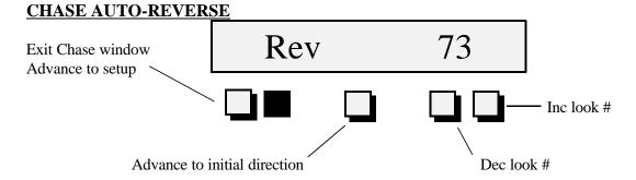
This parameter allows the chase to auto-reverse after a selected number of sequence loops. any number higher than zero determines the number of chase loops until the chase reverses direction. Next select the initial direction of the sequence by depressing the center button. Default value is 0.
