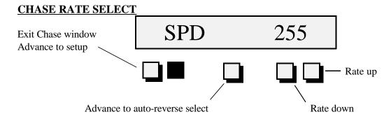
This parameter controls the relative speed of the chase i.e.: the rate at which the looks are sequenced. Depressing one of the two buttons on the right decreases or advances the speed. The rate can be programmed from "1" (fast) to "255" (very slow). Once the desired speed has been selected, depress the center button to advance to the next chase parameter. Default value is 5.
