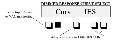
The curve select function allows users to accommodate a wide variety of lighting fixtures, special effects lighting, motor control, fluorescent/ballasted loads and more. The installed firmware provides for IES or linear curves. future software upgrades to accommodate other "preferred" curves may be installed based on your request. The above display represents a dimmer curve set for IES "Square Law" (preferred lighting curve).
