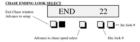
This display indicates the last step or ending look of the chase. Once again, depressing one of the two buttons on the right will change the last look #. After the last look has been selected, depress the center button to select the rate at which the sequencer will operate.
