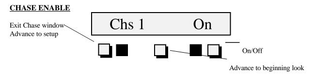
To enable the selected sequence depress the button indicated above. When a chase is active an <A' will be displayed next to the selected chase program as described in previous window.
