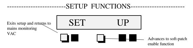
The SETUP function is used to access and select DMX patch on/off and slave on/off displays, analogue input on/off, pre-heat on/off, temperature °F or °C, regulation on/off, curve select IES/LIN, filter on/off, and lock on/off. Depressing the center button will display the soft-patch enable function. This setup menu may hold future software revisions/upgrades based on user requirements. Contact factory for update revision level.
