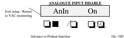
This function simply turns on or off the analogue control input to the dimmer. Default setting is "on".
