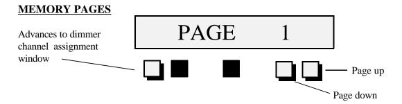
The PAGE features is a vehicle for storing and selecting operational functions such as; regulation on/off, preheat on/off, temperature  $\circ$ F/ $\circ$ C, filter on/off, analogue input on/off, dimming curve IES/LIN, soft patch on/off, and DMX assignments. These functions are located in pages 1 through 5, page 0 has been reserved as a location for slave addressing via remote dx units (see SLAVE function in SETUP menu).
