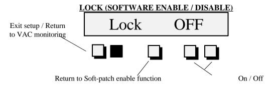
The lock feature enables all the programmed parameters in pages 0 - 6 to be locked out from any changes in all menus and set-up functions. When enabled, all parameters will be displayed in the main menus, but programming or changing will not be allowed. This feature is useful for rental companies to prevent the customer from changing pre-defined parameters. This feature has been provided as a redundant means to disable unauthorized use of controls. SEE "MODE SELECT SWITCH".
