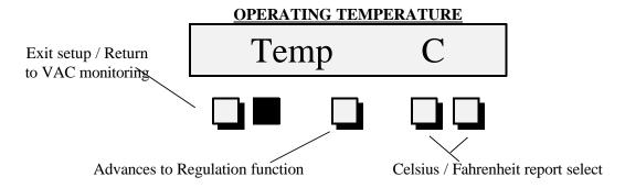
This display indicates the internal operating temperature of the unit. the temperature can be displayed in Fahrenheit or Celsius. to change the display, depress the far right or left buttons to change from Fahrenheit to Celsius. Default setting is F.
