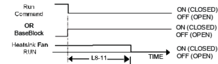
Figure 5.49 Heatsink Cooling Fan Operation Timing Diagram
