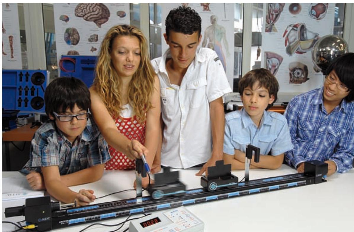
▲ Elastic collision study between two carts using the Timing set
