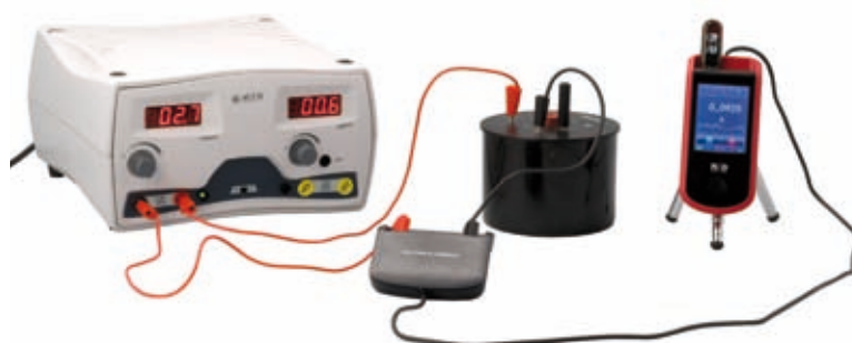
Experimental verification of the Joule's law with a RED Voltage & Current
