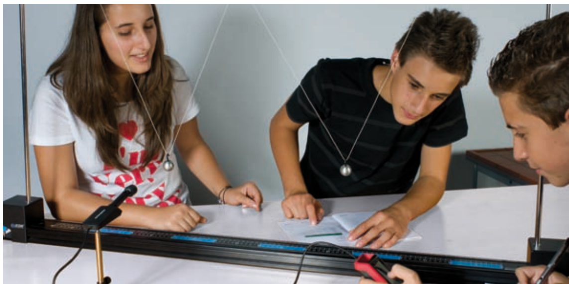
▼ Resonance oscillations between two coupled pendulum bobs
