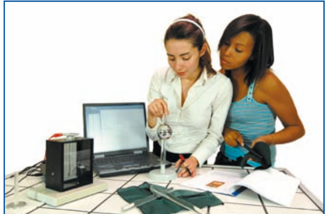
▲ Measuring charge in a hollow sphere with electroscope and datalogger
