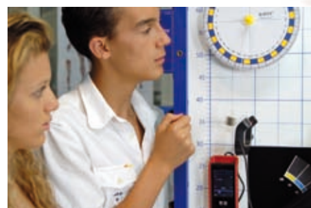
◀ Pendulum period measurement with a RED Photogate Sensor
