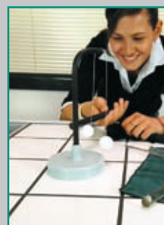
▶ Charging the electroscope by conduction
