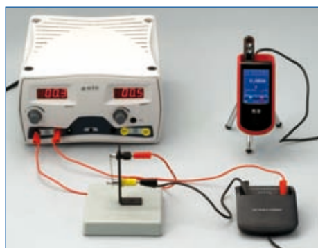
▲ RED Voltage & Current Sensor and Bimetallic Strip as a Thermostat
