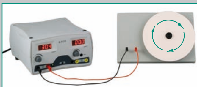
▲ The Newton's Disk consists in a disk with coloured segments printed on it, mounted on a base equipped by two safety sockets for connecting the power supply
