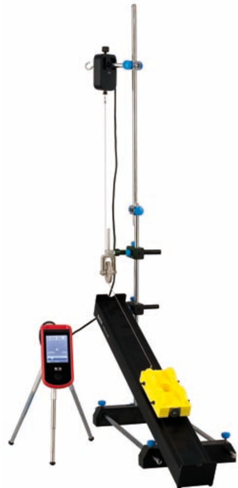
▲ Study of the tangential component of the weight force with an inclined plane and a Force Sensor
