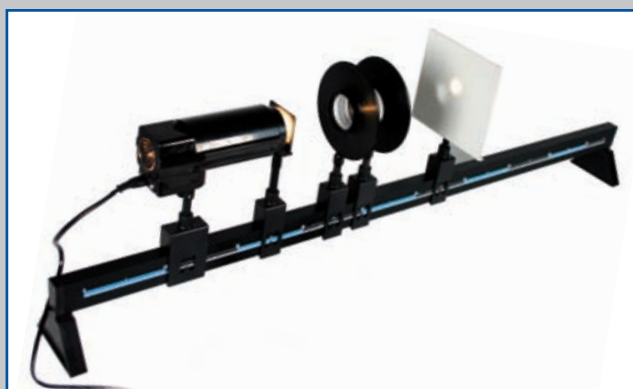
▲ Assembly for the determination of the focal length of a converging lens
