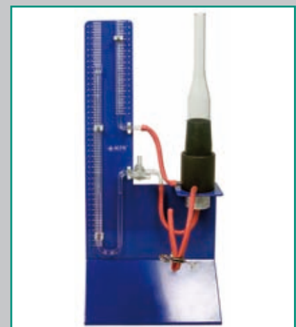
Thin shape vessel with 28 cm water height shows the same 13 cm pressure column height ▼
