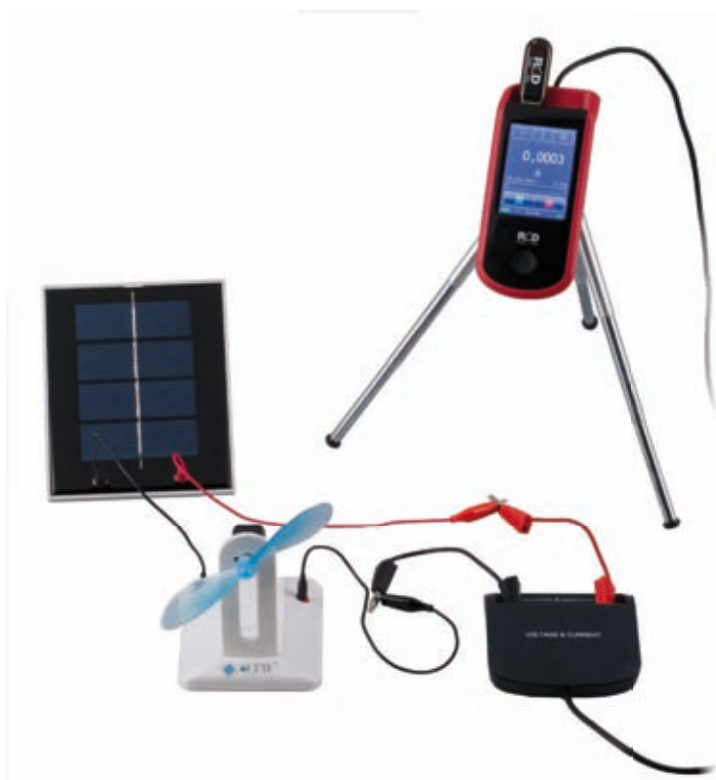
▲ Measuring the current produced by a photovoltaic panel
