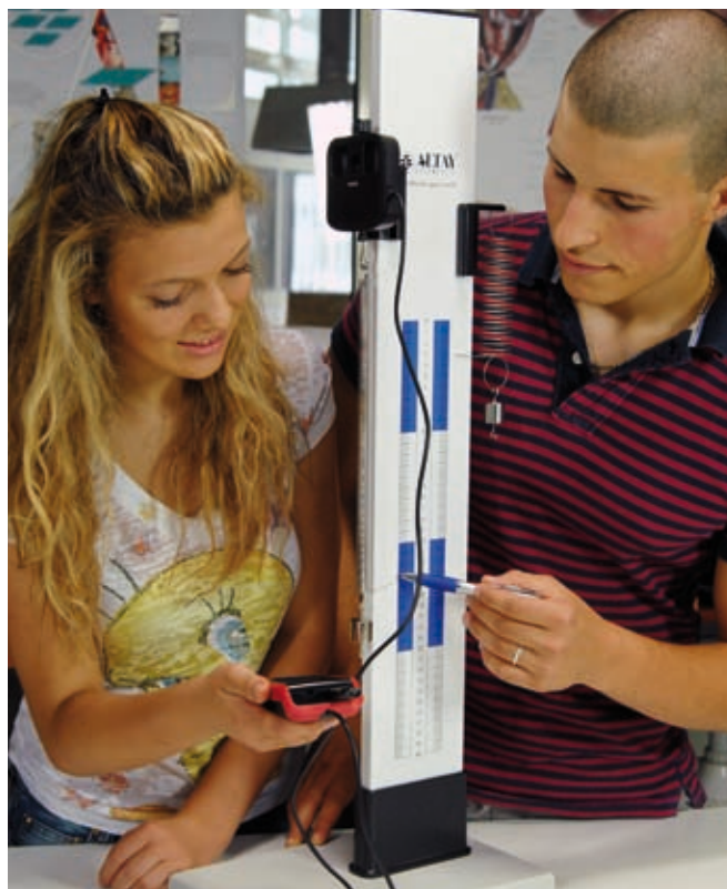
▲ Measuring the elastic force with RED Force Sensor
