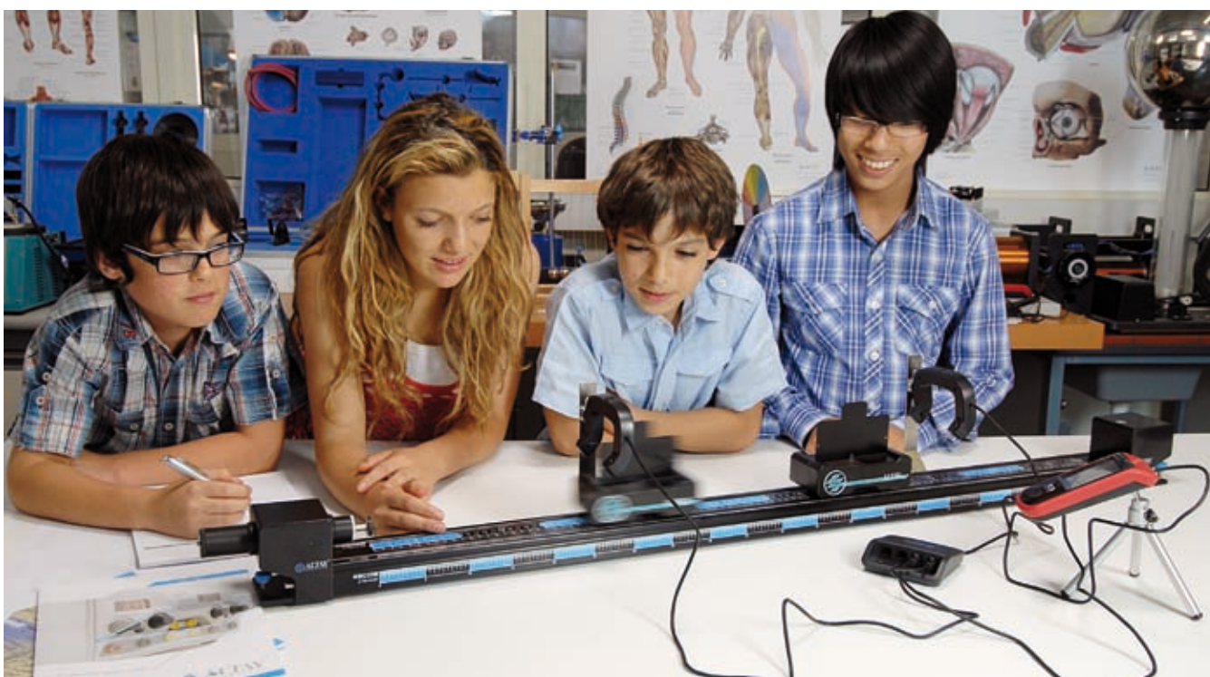
Elastic collision study between two carts using RED Photogate ▼
