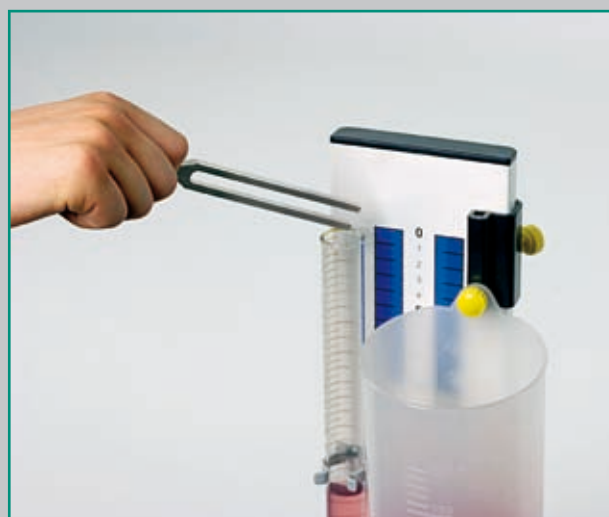
▲ The resonance tube matching the wavelength of the incoming sound wave
