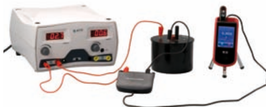
Joule's Law experiment with a RED Current & Voltage Sensor ▼
