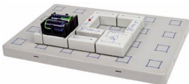
▲ Circuit setup for a current amplifier using a NPN transistor
