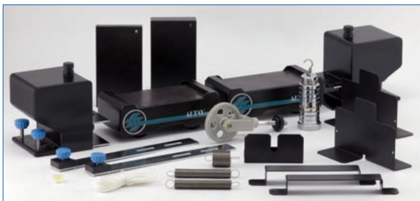
Elastic collision study between two carts using RED Photogate ▼
