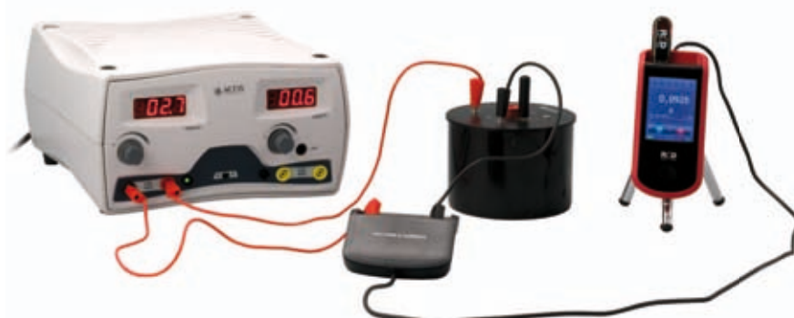
◀ Mixing calorimeter experiment with a RED Voltage & Current Sensor
