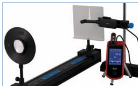
◀ Focus of a convergent lens using a RED Light Sensor
