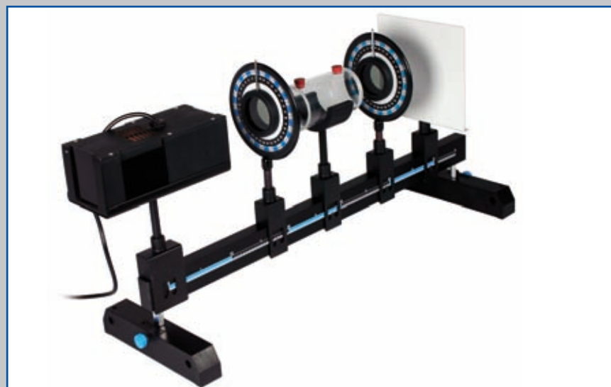
▲ Optics system 2 experimental setup to show rotation of light using a sugar solution
