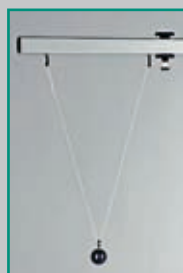
▲ Pendulum detail with bifilar suspension
