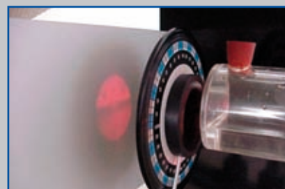
▲ For a given angle, all the polarised light is collected on the screen
