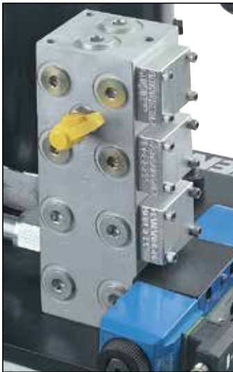
Attached manifold with 1 valve.
