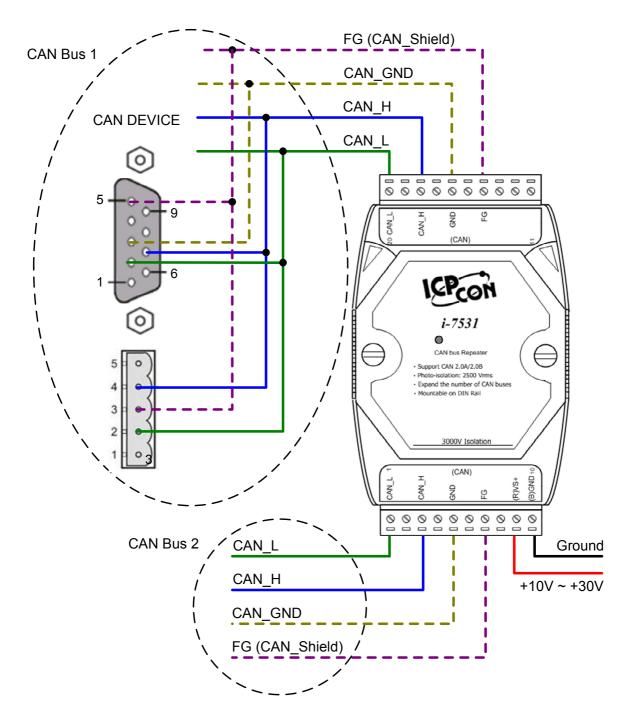
Note: Roughly speaking, wiring of CAN\_GND and FG between CAN devices can improve the capability of anti-interference of CAN bus system in harsh environment, but this is not necessary.
