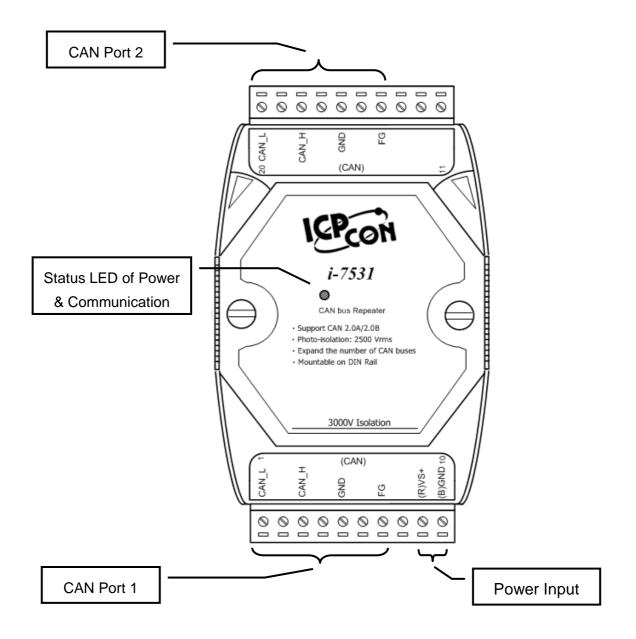
When the i-7531 is turned on, the status LED will be display with red light. Moreover, when a message passes through i-7531, the status LED will be twinkle once with yellow light while the red light is still on.
