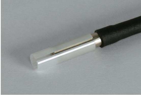
Figure 1 Insert the Mating Sleeve 1/2 to 2/3 of the way onto the Ferrule End of the Patch Cable
