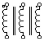
This component provides two or more coupled inductors. Electrically, it is equivalent with a vectorized Inductor (see page 81). In contrast to the vectorized Inductor, this component displays the individual inductors in the schematic as separate windings.
