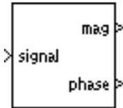
This block calculates the discrete Fourier transform of a periodic input signal based on discrete samples. The sample time, the number of samples and the harmonic order(s) can be specified. The fundamental frequency  $f_1$  of the running window is
