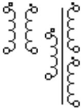
This component represents a transformer with two or more ideally coupled windings. At all windings  $w$ , the voltage  $v_w$  across the winding divided by the corresponding number of turns  $n_w$  is the same:
