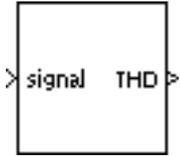
This block calculates the total harmonic distortion of a periodic input signal based on discrete samples. The sample time and the number of samples can be specified. The THD is defined as
