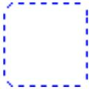
The Heat Sink absorbs the thermal losses dissipated by the components within its boundaries. At the same time it defines an isotherm environment and propagates its temperature to the components which it encloses. To change the size of a Heat Sink, select it, then drag one of its selection handles.
