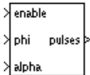
This block generates the pulses used to fire the thyristors of a 6-pulse rectifier or inverter. The inputs of the block are a logical enable signal, a ramp signal  $\varphi$  (produced e.g. by a PLL), and the firing angle  $\alpha$ .
