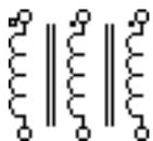
This component implements a magnetic coupling between three separate windings. For all windings the self inductance and resistance are specified individually. The mutual inductance and resistance are modeled as linear elements.
