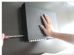
③ connect hard disk and mother board
