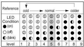
\* At level 2,4,6,8 the LED which is marked with ( $\bigcirc$ ) will light up fully ( $\bigcirc$ ) after blinking for 5 seconds.
