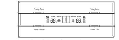
**Freezer Temp** : Indicates the current freezer temperature. **Fridge Temp** : Indicates the current fridge temperature.
