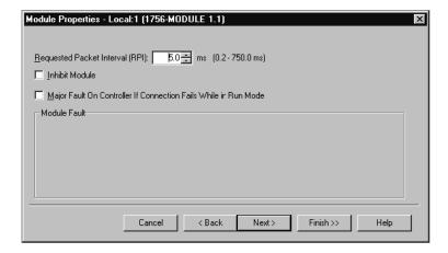
Select the Request Packet Interval value for scanning the I/O on the module. This value represents the minimum frequency the module will handle scheduled events. This value should not be set to less than 1 millisecond. Values between 1 and 10 milliseconds should work with most applications.
