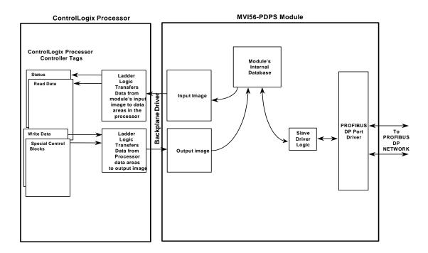
As shown in the previous diagram, all data transferred between the module and the processor over the backplane is through the input and output images. Ladder logic must be written in the ControlLogix processor to interface the input and output image data with data defined in the Controller Tags. All data used by the module is stored in its internal database consisting of 200 registers for I/O and Status information.
