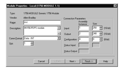
Fill in the dialog boxes as shown adjusting the Name, Description and Slot options for your application. You must select the **Comm Format** as **Data - INT** in the dialog box. Failure to set the **Assembly Instance** and **Size** values correctly will result in a module that will not communicate over the backplane of the ControlLogix rack. Click Next to display the next dialog box:
