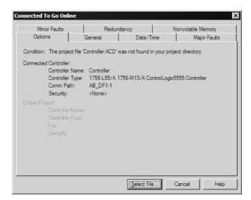
5 On the Connected To Go Online dialog box, click the General tab. This tab shows information about the processor, including the Revision (firmware) version. In the following illustration, the firmware version is 11.32
