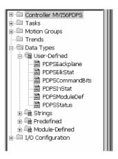
The next step in module setup is to define the data to be used to interface with the module and the ladder logic. Open the Controller Tags Edit Tags dialog box and enter the values shown in the following example. The MVI56-PDPS module is defined in the example as PDPS. You can set the tag name to any valid tag name you desire. If you are using the example ladder logic, this step has already been performed.
