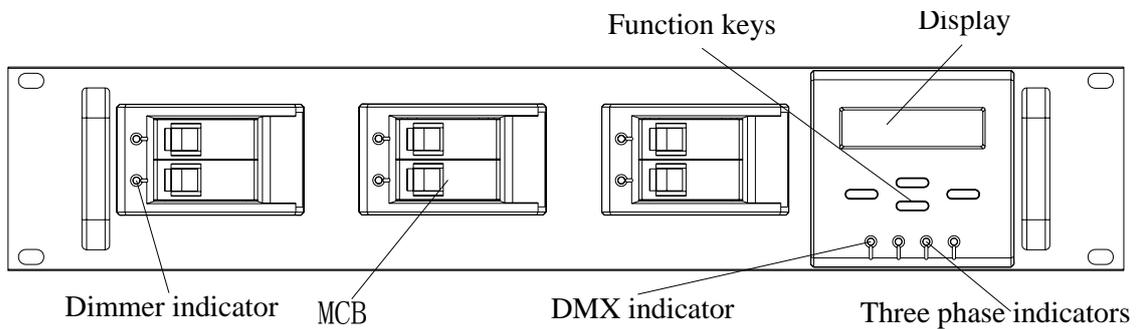
Function keys: consisting of 4 keys in total, namely "SETUP", "ENTER", "△", "▽".
