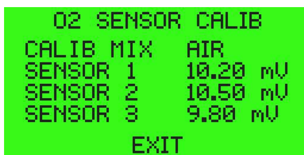
Figure 7: Calibration Screen (Calibration with AIR)
