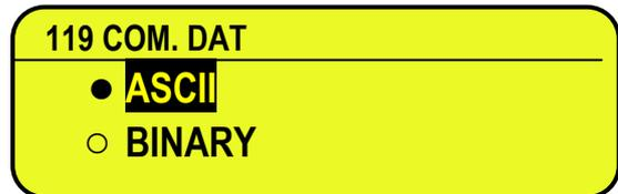
In the first screen one selects the port on which the diagnostic control should be executed. While in the second screen, one selects the code that one wants to use for viewing the data in transit.
