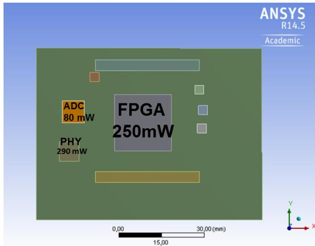
Picture 7 Power dissipation on the baseboard
