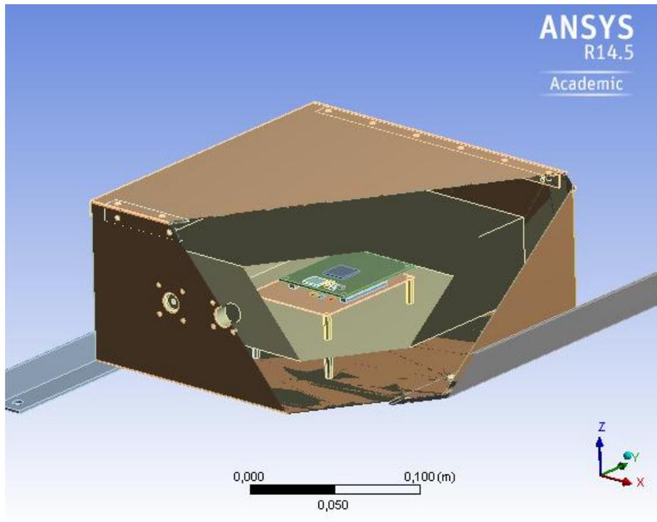
**Picture 2 PCB mounting in the experiment case**
