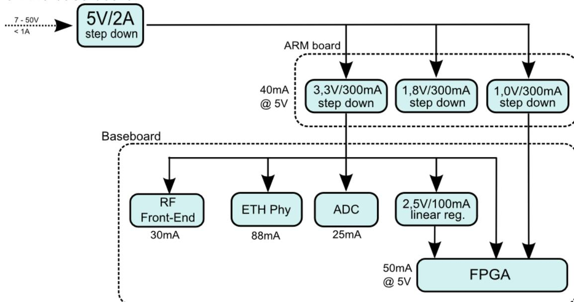
Figure 5 Power supply concept
