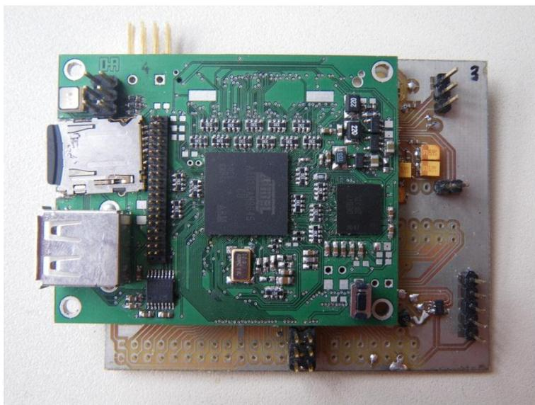
**Picture 4** Picture of existing ARM SoC board, including an old base board
