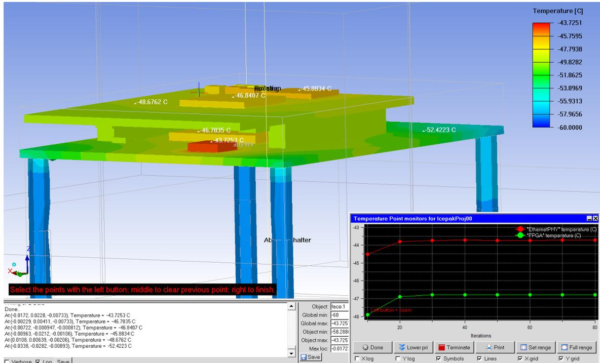
**Picture 6 Static Simulation Result of  $-60^{\circ}\text{C}$  environment, near vacuum**
