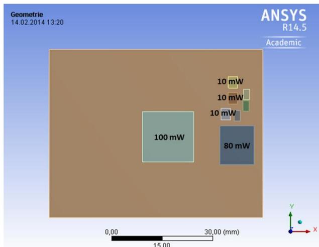
Picture 8 Power dissipation on the ARM Computer Board
