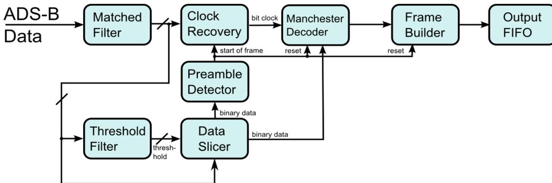
**Figure 6 Signal processing concept**
