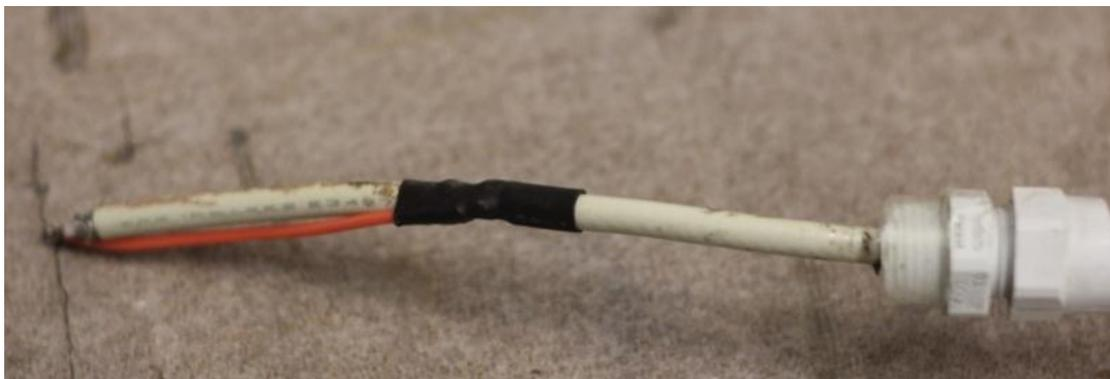
**Picture 14: Broken antenna after the flight.**
