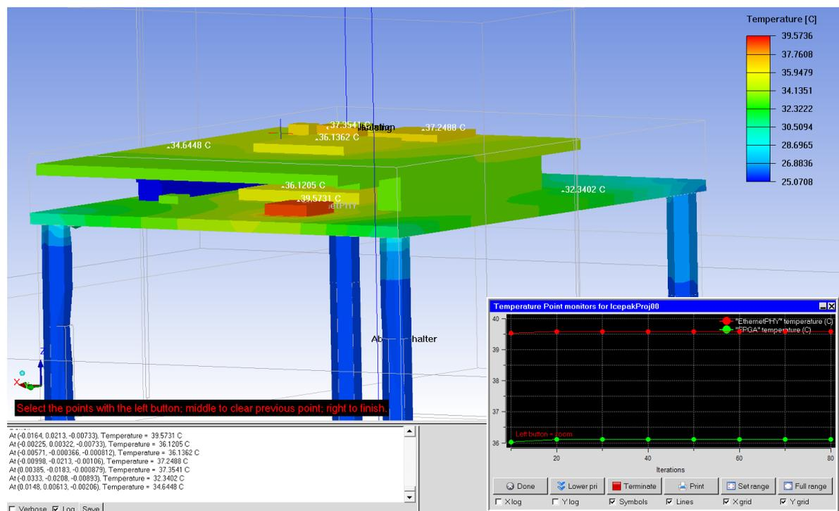
**Picture 5 Temperature profile of simulated vacuum test**
