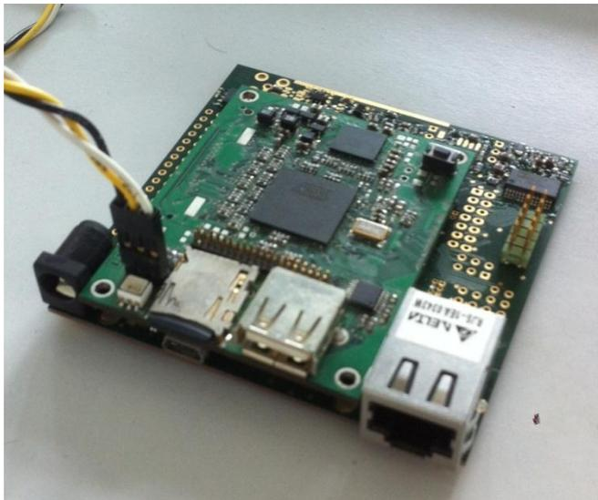
**Picture 5** The built ARCA baseboard (bottom) with ARM-board (top)
