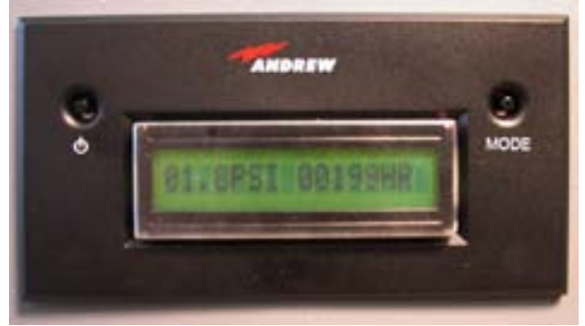
Mode 2: Displays pressure and total run hours, flashes current condition.
