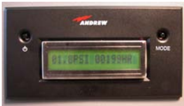
Mode 1: Displays pressure and total run hours.
