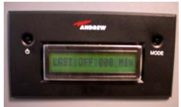
Mode 3: Displays last ON and last OFF times.
