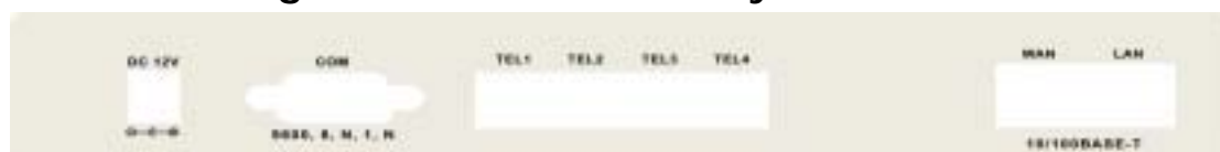
Figure 1-6 4AFXS Gateway Back Panel Ports
