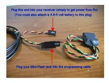
**Step 3:** Connect the POWER end of the programming cable (female plug) to your receiver and be sure the receiver is powered up (this connection to the Receiver simply provides power to the Mini-Flash during the downloading process; you could always use a 4.8v-5v battery instead of connecting it to your receiver)
