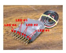
The picture to the left indicates the LED channel outputs. Notice that each of the 4 channels has two outputs, allowing you to connect two LEDs per channel. Add more LEDs to a channel by using a "Y" adapter or simply solder multiple LED lead wires onto the connector. As shown in the picture, the pins along the top are ground (-) while the pins along the bottom are positive (+).
