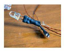
Only apply heat shrink around the metal portion of the connectors and connecting wires, especially on the connector side that will connect to the Mini-Flash controller (see picture). Also notice that this LED harness has female connectors on both sides. This allows you to replace LEDs (i.e. change a color). The LED connectors include a 100 ohm resistor (inside the black heat shrink tubing).
