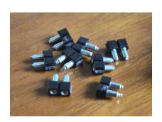
The LED mating connectors supplied provide a nice tight connection to the LED connector pins located on the Mini-Flash. If you are going to heat shrink these ends, be sure you do not cover the black portion of the connector as this will not allow you to plug these connectors side-by-side onto the Mini-Flash (heat shrink makes the connectors too wide). If you are only using 4 LEDs (one per channel), then you can skip every other connector.
