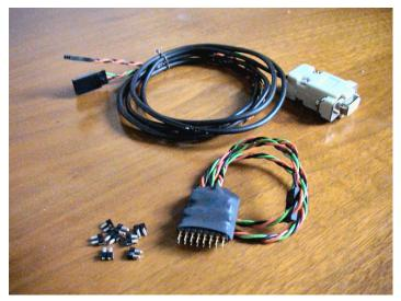
The picture to the left indicates exactly what is included in the Mini-Flash kit: (1 controller, one programming cable and eight 2-pin LED mating connectors). Remove the contents from their plastic packing bags and be sure to not loose the small miniature LED mating connectors. These connectors mate to the controller's LED connections. To use these connectors, you will need to solder on some small gauge, two conductor wire, a series resistor (see below) and finally your
