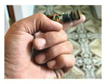
Weighing merely 9 grams and roughly 1 square inch by 1/4" thick, the Mini-Flash is based around a tiny 8-pin programmable microcontroller chip. The controller can gets it power from either an R/C receiver or an external battery (normally, it is plugged into a receiver). The Mini-Flash is designed to operate off of a 4.8-5 volt power source therefore do not attempt to run it off of anything else or you will ruin the microcontroller. The Mini-Flash
