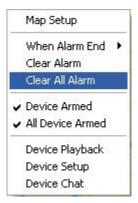
User can choose *Clear Alarm* to clear the kept alarm for the device or click *Clear All Alarm* to clear alarm for all devices.
