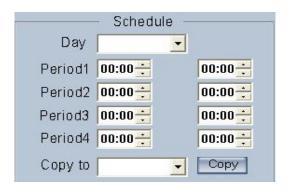
【Copy to】 After finishing one channel, if you want to set any other channels' configuration as the same as this camera, you can select channel number from drop-down list, and press Copy button.
