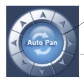
Pressing this button initiates the connected PTZ camera to do an automatic tour of 360°.
