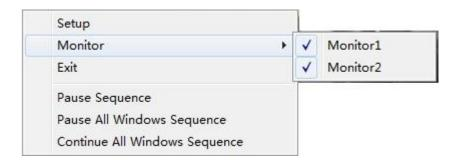
All the monitors connected on the TV client PC will be listed there if you click "Monitor". Select one monitor to hide it. If you don't check "Monitor 2" here, then, the monitors will turn to like this (The second monitor displays the desktop only.):
