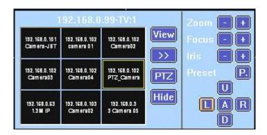
PTZ can only be controlled when PTZ camera is selected. It's nearly the same with the operations on PTZ control panel. But you can only call the preset you have set. You can't set the preset here.
