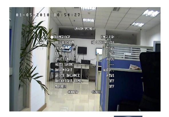
When you enter the menu, you can control it by down, using up, down, left and right buttons. Press IRIS – ( ) to enter the sub menu. When you use up or down to move to "exit", press IRIS- to exit the menu.
