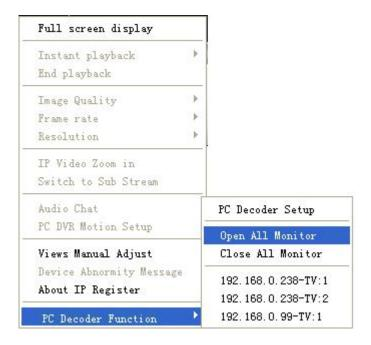
Select "Open All Monitor" in right click menu to view all the monitors connected in the system. You can drag them to anywhere. The names of current display cameras on TV client will be shown in the monitor window.
