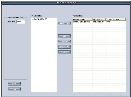
The IP "192.168.0.99" here is one of the PC you installed TV client on. After you filled the CMS IP "192.168.0.192" (the sever end, mentioned before) in login interface when running TV client, its IP will be displayed here automatically. Click "Add" button to add it to the Monitor List so that you can setup it later.
