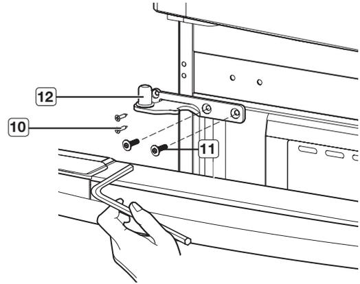
2. Place the hole in the bottom of the door over the lower hinge(**12**).
