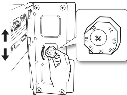
Example) The slope is about 2mm (0.08inch) as shown below.
