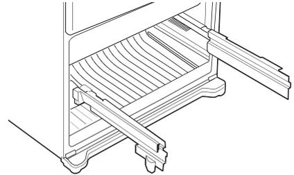
2. Attach the freezer door front onto the open slots on the sides.
