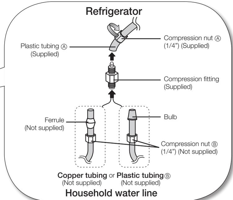
1. Slip the compression nut ① through the supplied plastic tubing ①.
