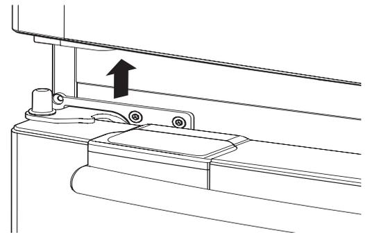
5. With a Philips head screwdriver, remove the two screws (10) attached to the lower left and right door hinges. With an wrench(3/16"), remove the two hex head bolts (11) attached to the lower left and right door hinges. Remove the lower left and right door hinges (12).
