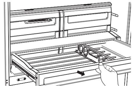
To remove the divider - Pull the pantry completely out to full extension and raise the front side of the divider to unhook it from the rear wall of the pantry, then lift the divider out.
