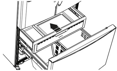
2. Remove the tilting pocket(1) by pulling on both brackets(2) upward at the same time.
