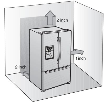
First thing! Make sure that you can easily move your Refrigerator to its final location by measuring doorways (both width and height), thresholds, ceilings, stairways, etc.
