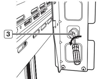
3. Find the best level to align the door slope.
