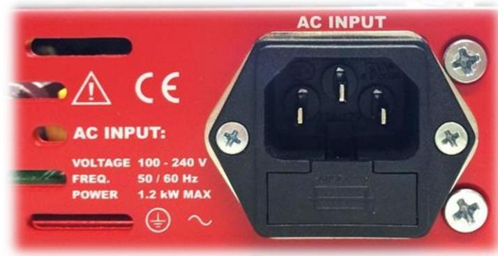
**Figure 3:** AC Power Line input socket
