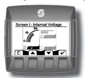
**3.** After screen type selection, select signals to monitor. Use the up and down arrow soft keys to cycle through available signal selections.
