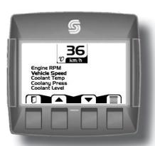
The Quick Data function allows selected signals to be monitored in a scrollable single view display.
