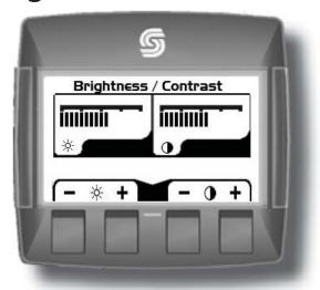
Adjust brightness and contrast levels by pressing the far left soft key. This will display the brightness and contrast soft key bar. The bar will disappear after 3 seconds of inactivity.
