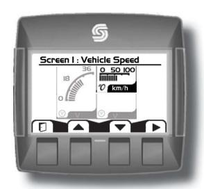
**4.** After making a signal selection, press the right arrow (Next) soft key to go to the next selection area. Use the up, down arrow, next and select soft keys to select signal. Select the right arrow soft key to move to the next selection area.
