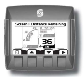
**5.** Using the right arrow soft key will rotate through the selections in a clockwise rotation.
