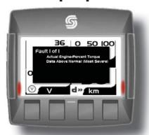
When a fault is detected on the CAN network, a flashing red warning alarm will be activated and a fault information pop-up window will be displayed listing current fault information.
