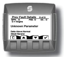
Selecting Previous Faults in the Fault Menu will display all previously active faults on the CAN network.
