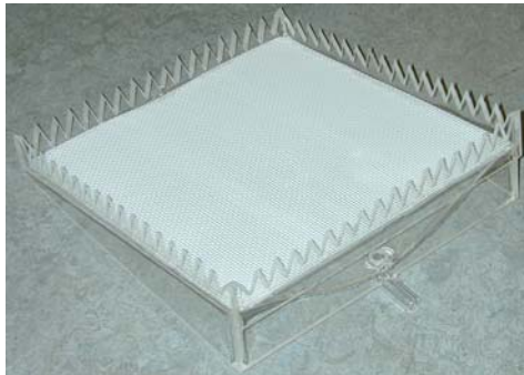
Figure 11. Percolation lysimeter (Note that the lysimeter drains freely through a tube connected to a 5-L collection container (poly-propylene), which is graded to allow the field recording of the collected volume.
