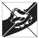
If the power cable wires are frayed or cut
