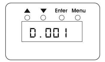
The UP/DOWN keys change the value for the start address. Watson uses the changed value immediately and permanently saves it after 10 seconds or if the Enter or Menu key is pressed.
