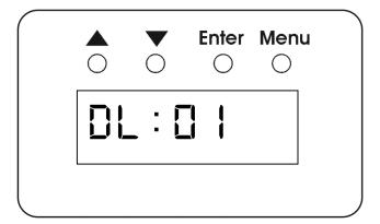
Delay times are represented in seconds, and can be set from 01 to 99 seconds.
