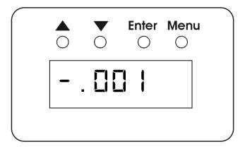
When valid DMX is detected, the dash is replaced with the letter 'd' for DMX:
