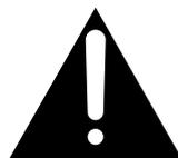
The exclamation point within an equilateral triangle is intended to alert the user to the presence of important operating and maintenance (servicing) instructions in the literature accompanying the appliance.
