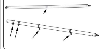
Then insert the tail boom into the tail boom holders (70-00093, 70-00094). Lock the tube in place with screw M3x8 (70-00086) via the clamp up and additionally with screw M3x6 (70-00053) as shown. Install the carbon support beams (70-00104-70-00106) on the main frame and the tail boom tail boom clamp (600UH1-007).
