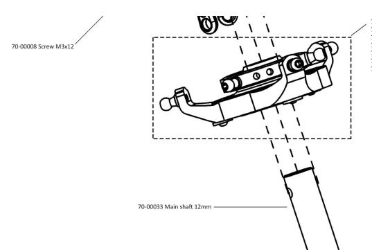
70-00026 Ball joint 22mm 70-00027 Swash upper ring 70-00028 Bearing 30x42x7 70-00029 Swash lower ring 70-00030 Uni link 5mm 70-00031 Washer 2x8x1 70-00032 Screw M2x6
