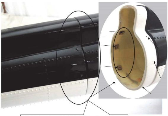
Drill six holes as shown to install the tail boom, then glue the wooden blocks 【40】 into the inside as shown. Do not mount the tail boom yet.
