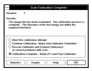
Selecting **OK** will start the process of making LFC's.
