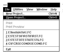
To manually open an existing project, select **O**pen Project from the **F**ile pull-down menu.
