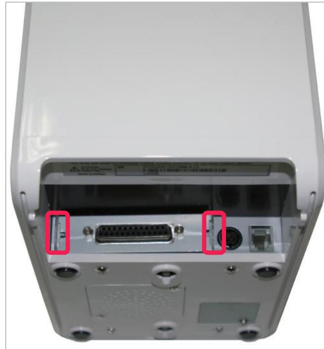
1. Remove screws from either side of panel as shown above.
