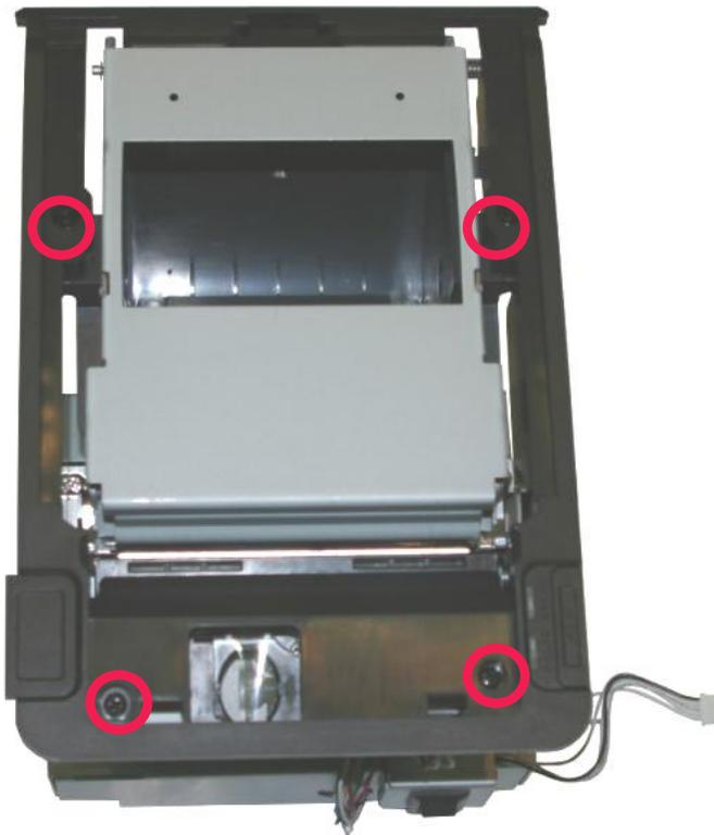
5. Remove all 4 screws from the cover of the printer. (2 metal screws from upper side and 2 black screws from lower side.)
