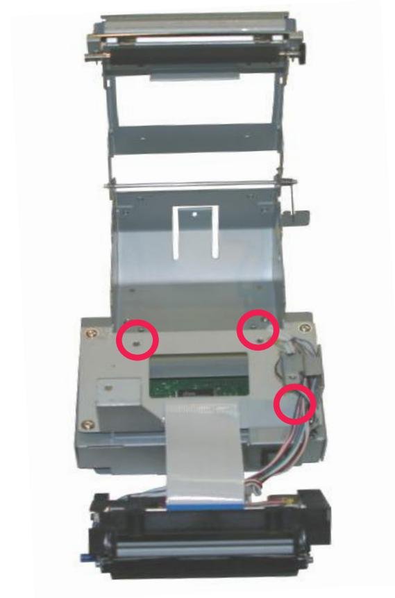
9. Remove the 3 screws from the areas shown above and disconnect data cable.
