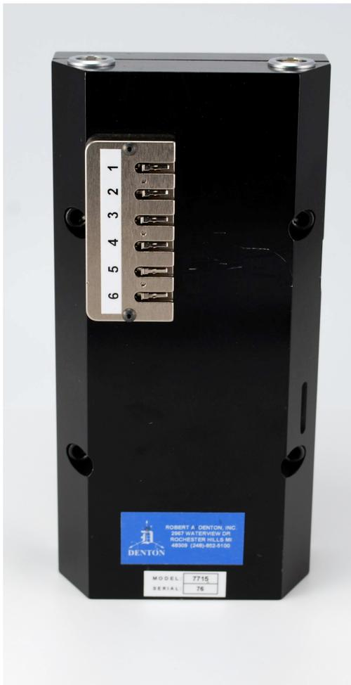
**Figure 1A. RibEye controller/sensor rear view**
