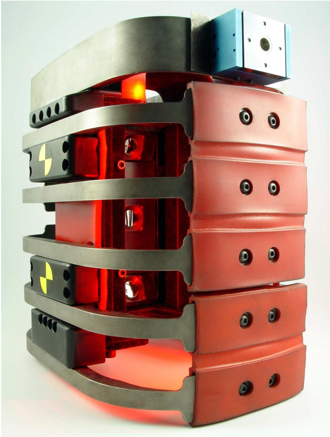
**Figure 6. RibEye controller/sensor mounted in the SIDII's thorax**
