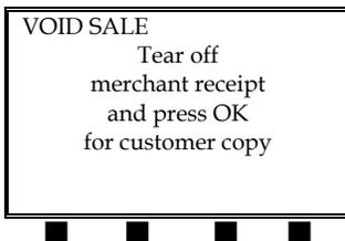
Tear off the merchant copy of the receipt and press [OK] to print the customer copy.
