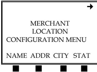
To enter the company name, press the [■] key under the prompt NAME, to enter the company street address, press the [■] key under the prompt ADDR, to enter the city name only, press the [■] key under the prompt CITY, to enter the two character state name, press the [■] key under the prompt STAT or press the [MORE] key to enter other merchant information.
