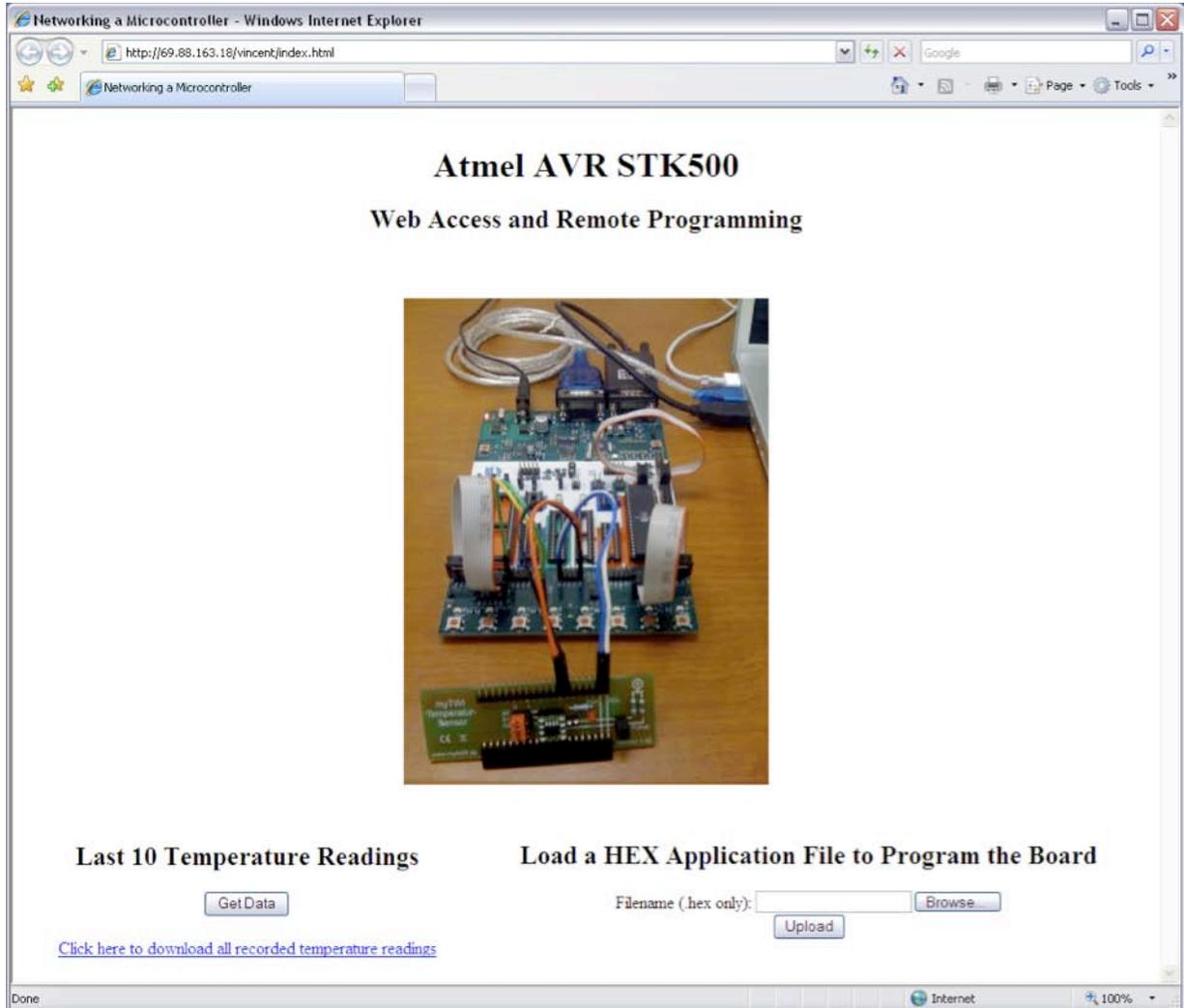
**Figure 4.46** Screenshot of the sample website used to remotely access the myTWI-to-STK500 data acquisition system.
