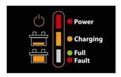
•Fully / Float: Battery is fully charged and is being maintained.
