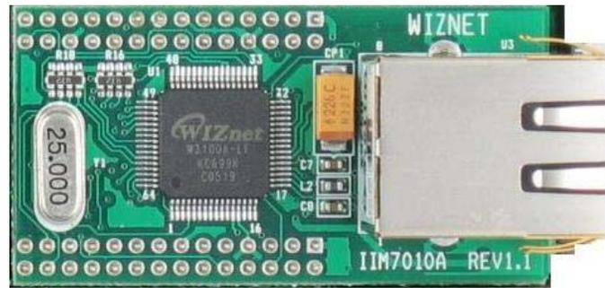
Figure 3.8 WizNet™ Ethernet Module
