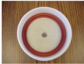
Figure 5-11: Disk Holder Cup with gasket
