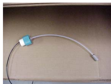
Figure 4-2: Bottle Cap Assembly with solvent filter
