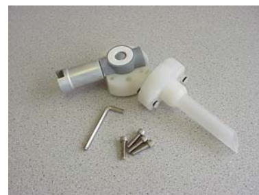
Figure 7-4: Inside the Water Inlet Valve
