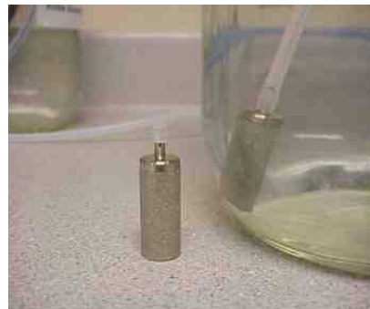
Figure 7-11: Inlet Solvent Filters
