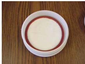
Figure 5-12: Disk Holder Cup with 3M Empore™ O&G disk.
