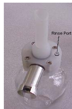
Figure 5-19: Water Sample Inlet Valve Rinse Port
