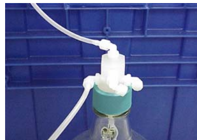
Figure 4-6: Solvent Waste Recovery Assembly
