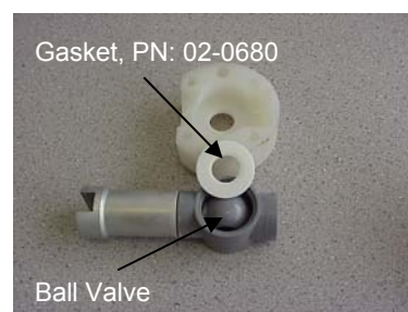
Figure 7-5: Ball Valve and gasket sealing
