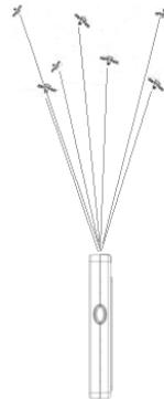
Always try to leave the antenna area free from metallic objects that obstruct GPS signals from the sky. Human body affects GPS signals, if *e-track<sup>TM</sup>* is being used to track a person, try to locate the unit above the person's waist to reduce the human-body signal-blocking. Outside pockets are better locations than inside (jacket) pockets. The best locations for person tracking are outside-jacket pockets and front-shirt pockets, having the LEDs' area on top (GPS antenna is in
