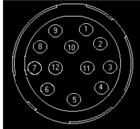
Front View of Connector of Sensor
