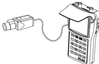
The working time of camera are different because of different consumption camera, it can work more than 4 hours if it work with a camera that consumption current is less than 100mA, The maximum output current from tester is 200mA, please use the proper camera to work with.
