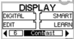
Advanced mode has four display options – SMART, DIGITAL, LEARN and EDIT. The DETECT shortcut button is used to cycle between them. Advanced mode's SMART and DIGITAL have the same screen elements and functions as those in Quickstart. For a refresher on this, turn back to pages 40-48 of Chapter 5: Quickstart.
