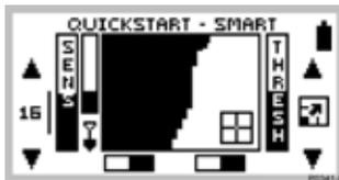
Figure 5.3 Smartfind display with preset Coins discrimination pattern
