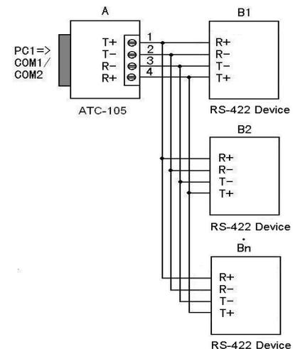
**5.3. Full duplex communication connection between ATC-105 interface converters**
