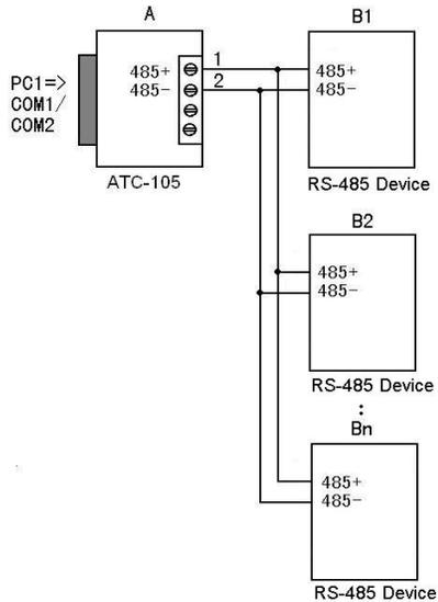
**5.6 Half duplex communication connection between ATC-105 interface converters**
