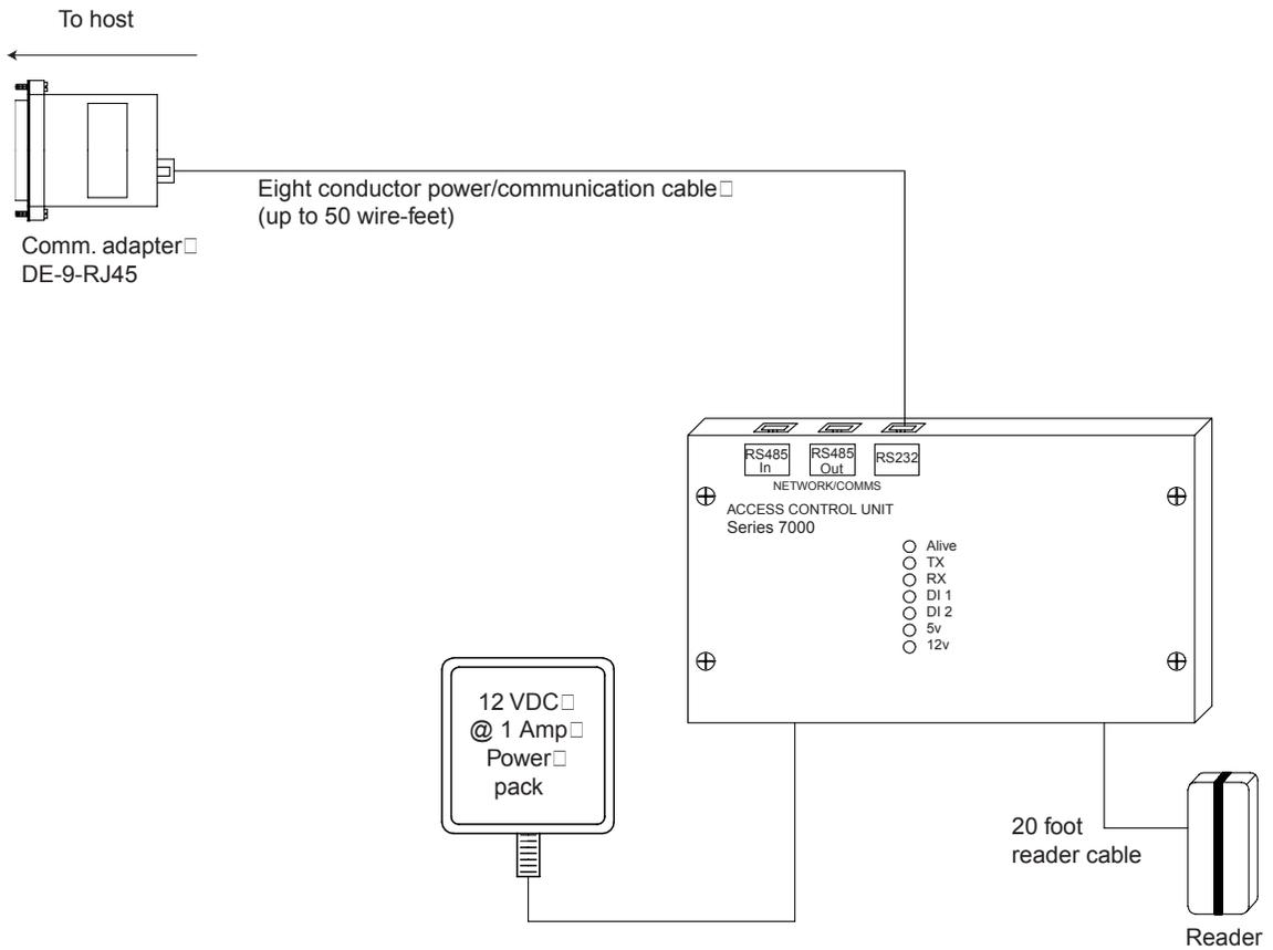
**Figure 2-8: Series 7000 RS485 Serial Installation**
