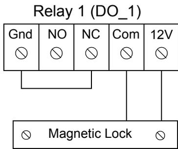
12VDC magnetic lock. Connection normally closed (powered to maintain locked state).
