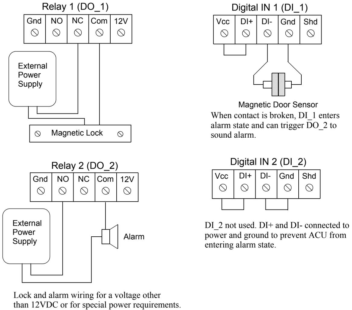
**Figure 2-6: Dual Door Mode Wiring Example**
