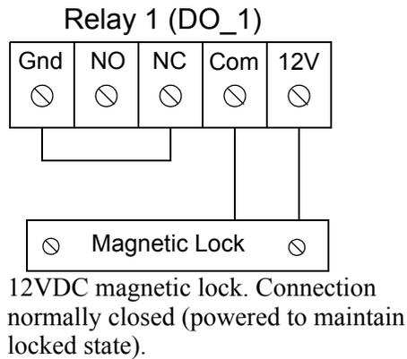
In that wiring example, the power for the door lock is being taken from the 12V terminal on DO\_1. [Figure 2-5](#) shows an alternative method of powering the door lock from an external source for a voltage other than 12VDC or if the lock requires more power than can be supplied by the 12V relay connection.
