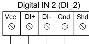
DI\_2 not used. DI+ and DI- connected to power and ground to prevent ACU from entering alarm state.
