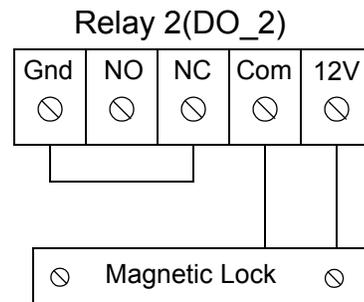
12VDC magnetic lock. Connection normally closed (powered to maintain locked state).
