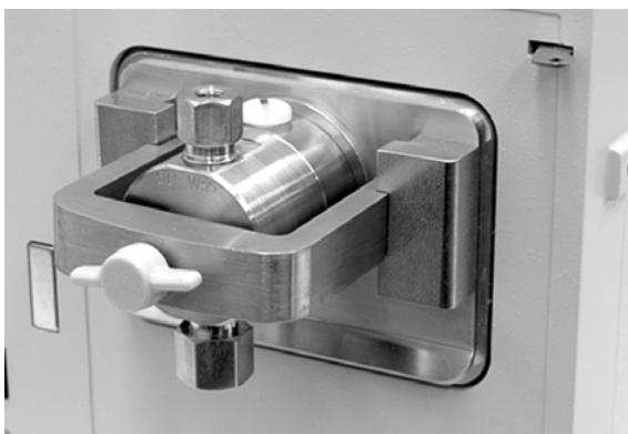
Figure 4 Pump head installed on the pump
