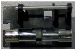
Figure 24 120 V fuse in holder
