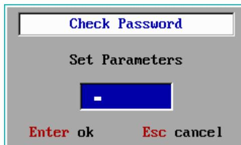
After inputting the correct password, press <Enter> key to enter Set Parameter menu.
