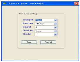
After connecting with communication box, computer auto identify relevant serial port; Baud rate is "115200", data bit is "8", check bit is "none", stop bit is "1". Click "sure".
