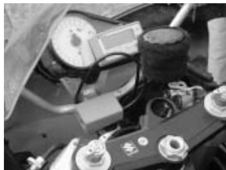
Poor mounting — although the Ultra-Lap is pointing toward the transmitter when vehicle passes, the receiver is too far "inside" the bike and does not have a wide view toward the transmitter.
