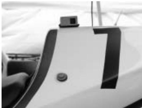
Good mounting on the tail section; clear and wide view toward the transmitter when the vehicle passes.
