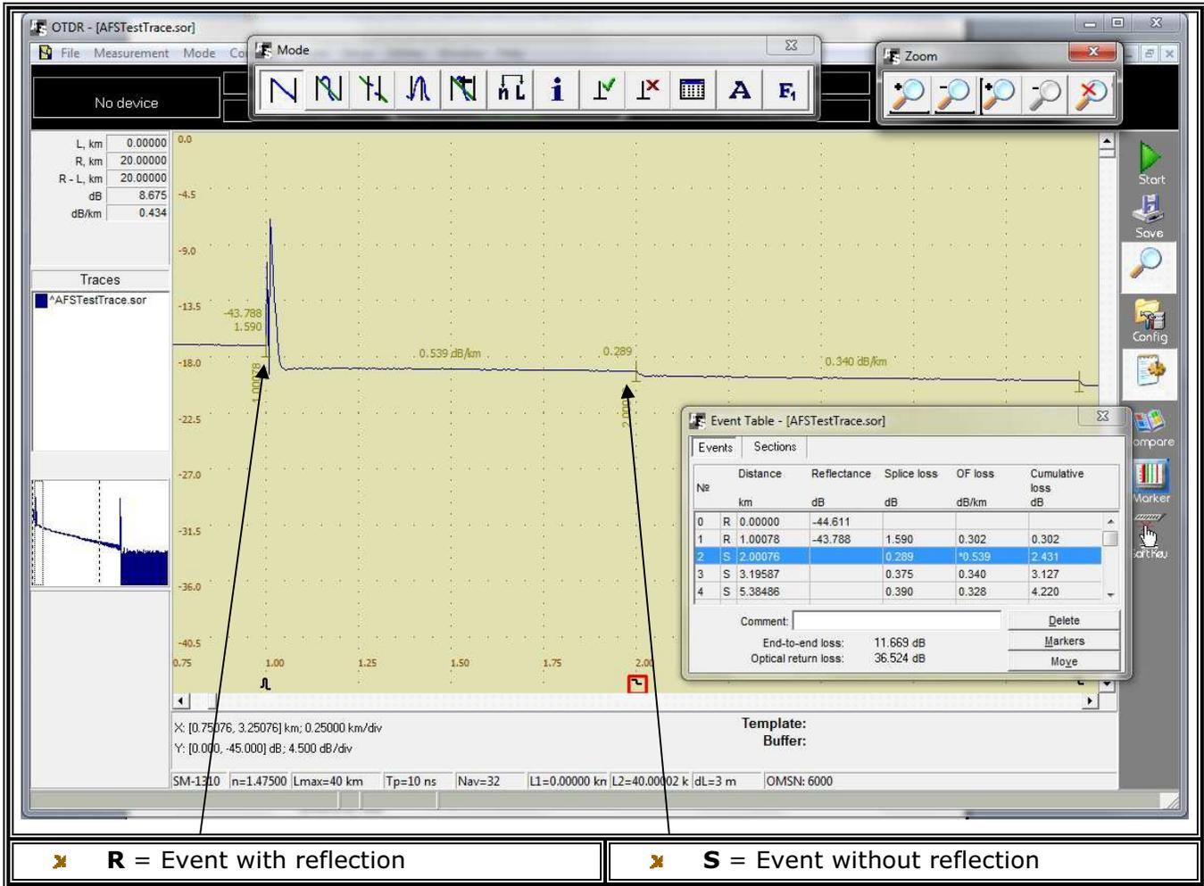
The **Events Table** lists the measurement values of the data points (marks, ⊥) on the particular fiber under test. The Events Table (**table 8.0**) has two fields, the "Events" field and the "Sections" field.
