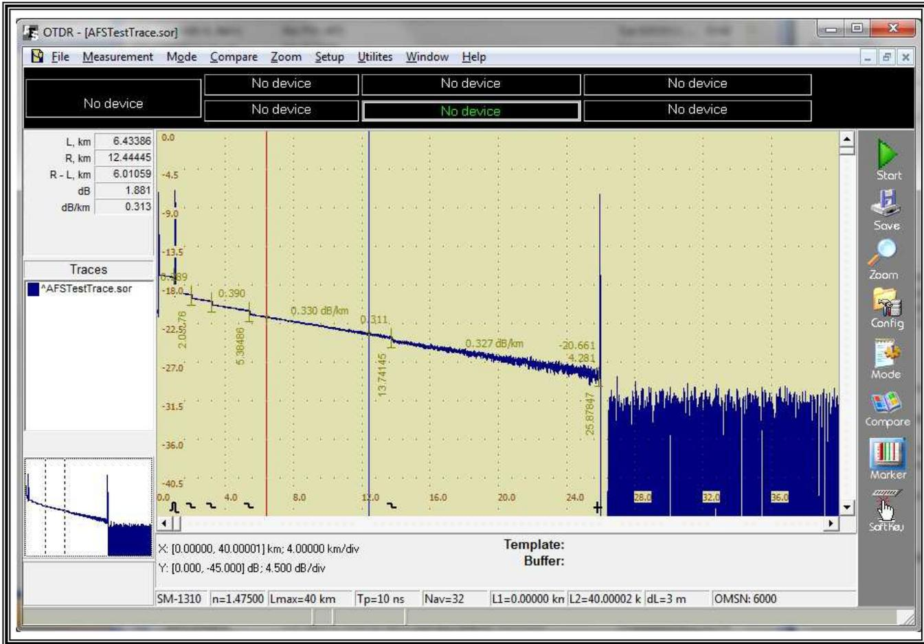
A Trace is a visual representation of a fiber optic link. The beginning of the fiber optic link is located on the left side of the trace. The slope or attenuation of the fiber link can be seen as the trace moves to the right. There are two “active” markers, the information containing the location of the markers is located on the left side of the screen as shown above in Table 3.0
