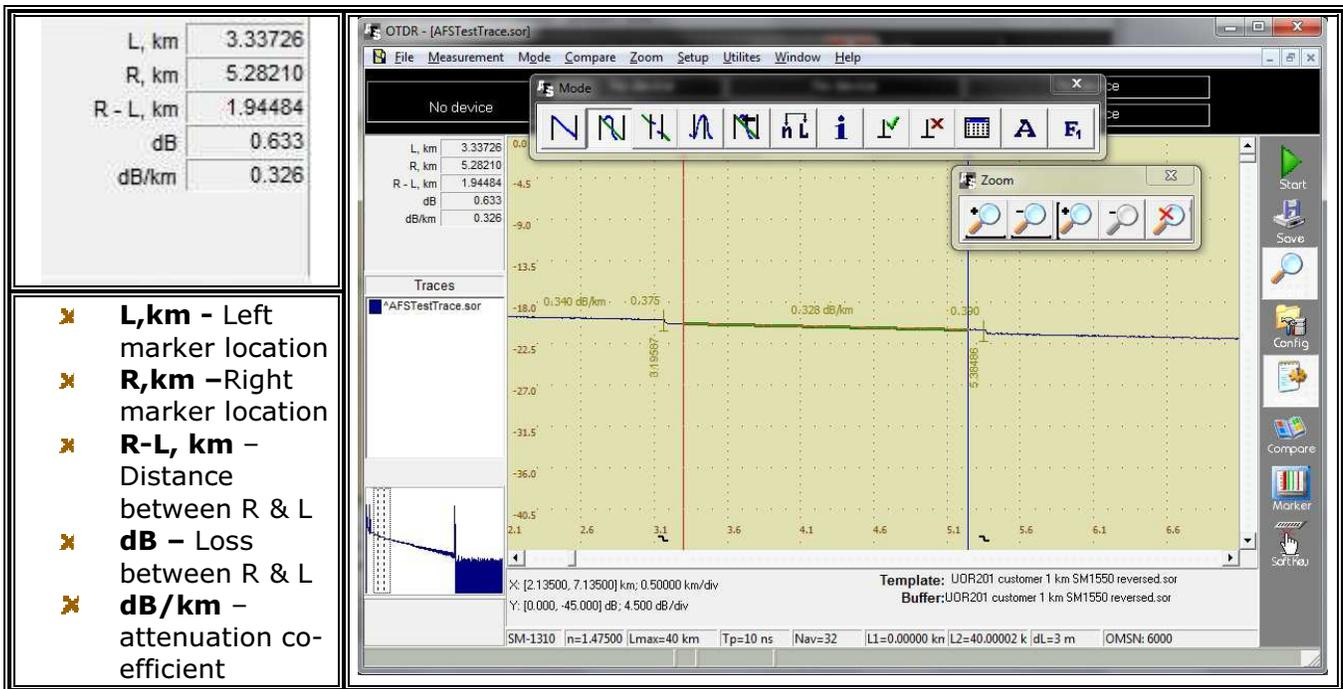
**\*15 Attenuation Measurement of an "Event" – (Splice Loss)**
