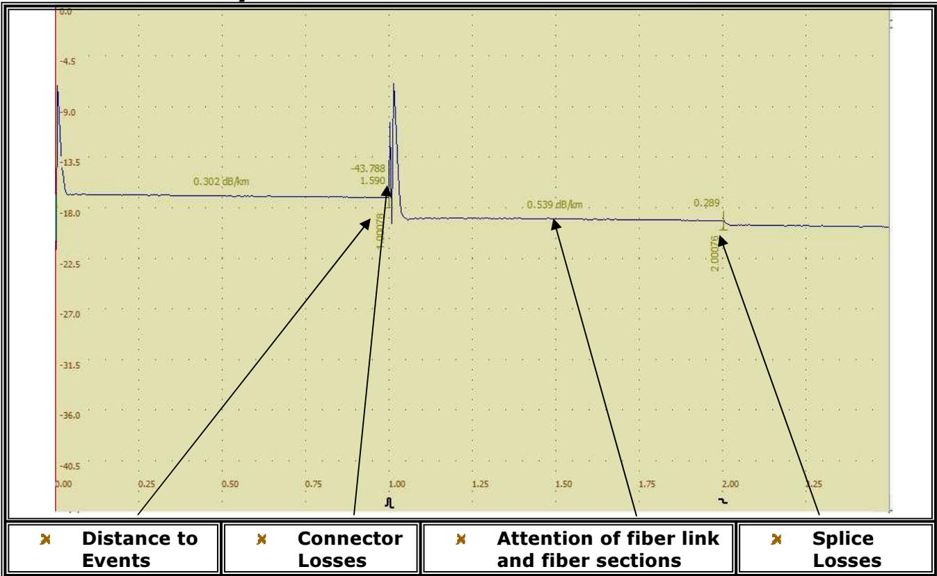
When the OTDR takes a measurement it also performs an automatic trace analysis (if preset). Once the trace analysis is completed, the OTDR will determine the following, the **distance** of the fiber link and **distance to events**, the **attenuation** of the fiber link and of fiber sections, the **ORL**, the **splice losses** and the **connector losses**.
