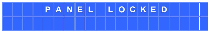
To re-enable the front panel controls, it is necessary to enter the stored password. To do this, access the lock menu (left and right PARAM keys simultaneously for 2 seconds). The following screen is displayed:
