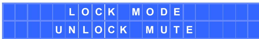
Using the rotary control, it is possible to change the desired locking mode and then press SHIFT + ENTER to confirm the selection. If you select one of the two password protected modes (LOCK ALL or UNLOCK MUTE), the next screen prompts you to enter the lock password:
