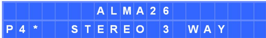
An asterisk to the right of the preset number indicates that it has been modified and not yet saved in the memory of the ALMA26.
