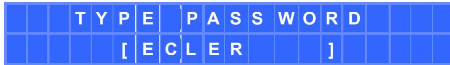
Using the rotary control, edit the selected character, and using the PARAM keys, select the next character to edit. Finally, press SHIFT + ENTER to validate the entered password.
