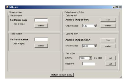
For calibrating the 4 mA point click on "Test" in the field "Calibrate 4 mA".
