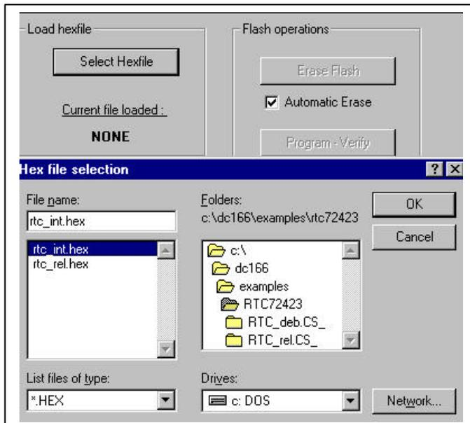
Now select the Flash operation Program – Verify, to download the project into the internal Flash. After a successful download, you have to switch OFF the BSL-switch S3-5, switch ON the single chip-switch S2-3, press the Reset push button S1 and start a terminal program on your PC with the line parameters 9600Baud, no parity, 8 bit data and 1 stop bit.
