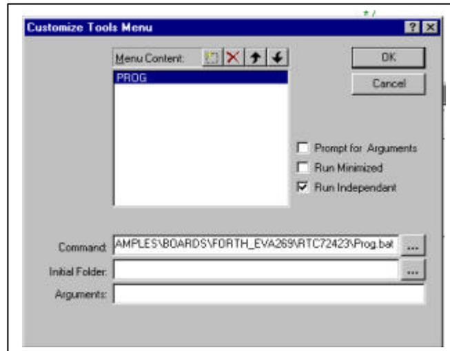
The batch-file "PROG.BAT" converts the hex-file of the project into a binary file, which will be downloaded into the external Flash, by the FLASH166 program.
