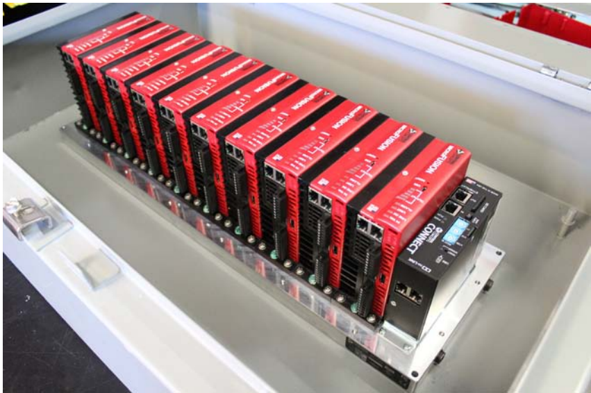
Figure 4: Mounting liquid cooled heatsink inside of an enclosure. Note: Liquid connections are not present in photograph.
